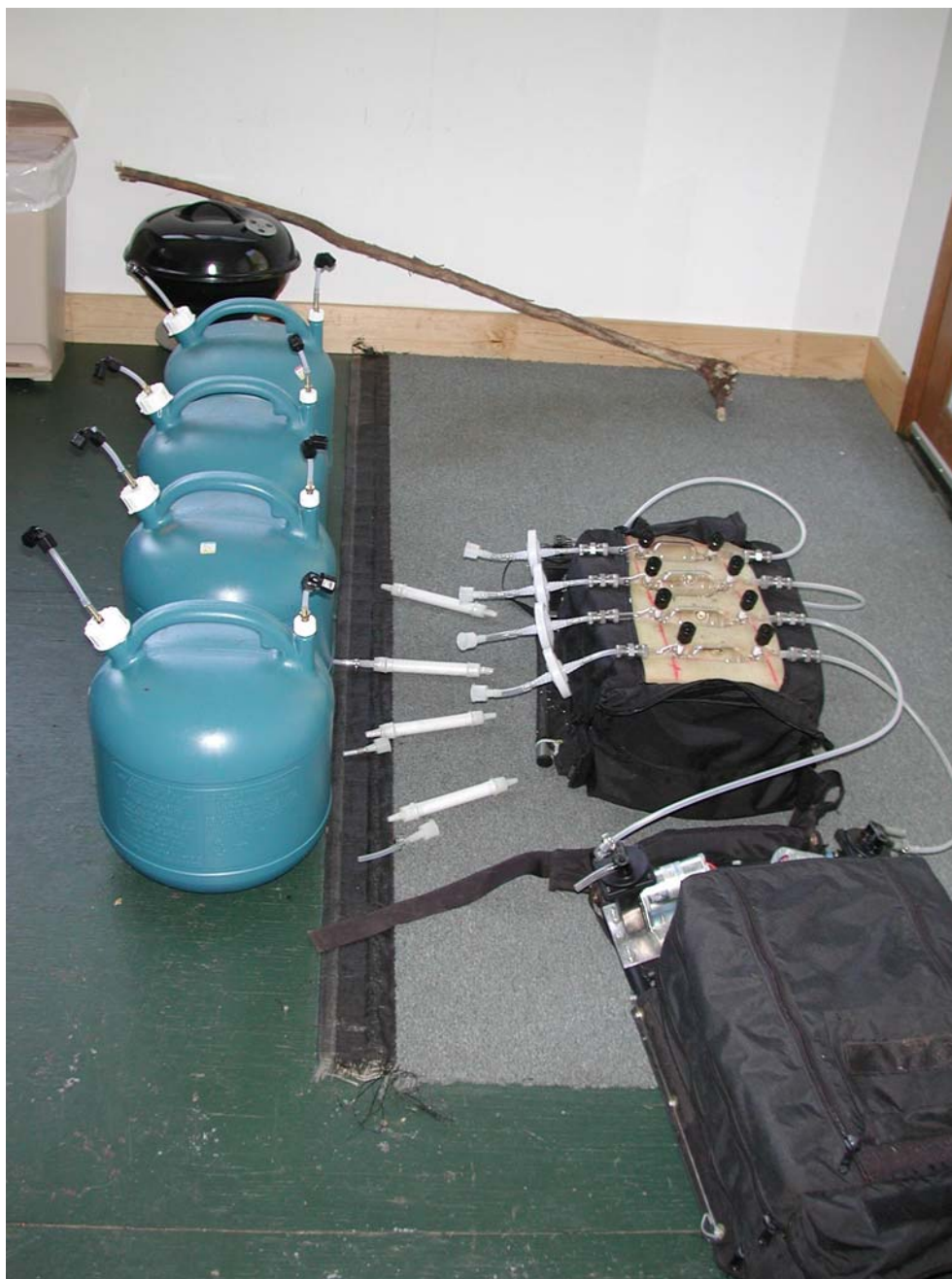
Figure 18. Stable isotope canopy profiling system with buffer volumes.
